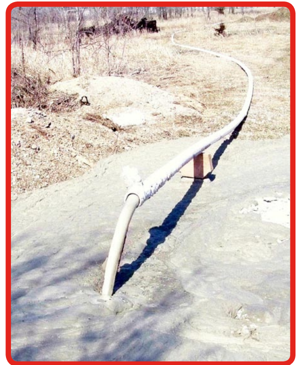
This photo shows one of the tests that Richway has done pumping 30PCF material through 1000’ of 3” PVC pipe. Richway has also performed similar testing with 2” hose up to 1000’ in length successfully
