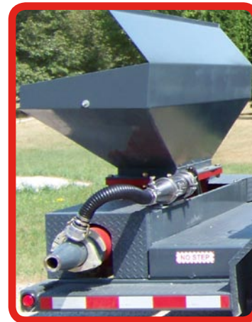
As seen in this photo the foam hose comes from the stainless steel Foamhead TM (where the foam is physically generated) and is connected to a machined injection barrel on the discharge side of the pump. Part of this assembly includes the static mixer
